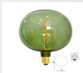
DT200-O 4W LED, DT200 Gradient Olive Spiral Filament, AC220-240VAC, Warm White (2800K) DIMMABLE
